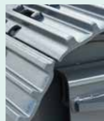
Increased shoe plate thickness
