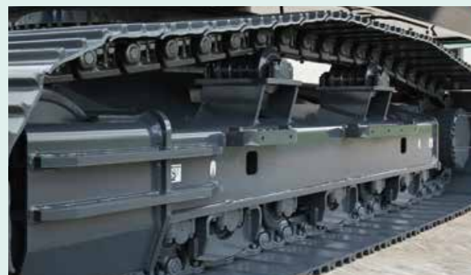
Track guides installed in three places
