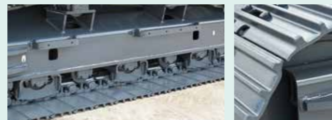
Track guides installed in three places
