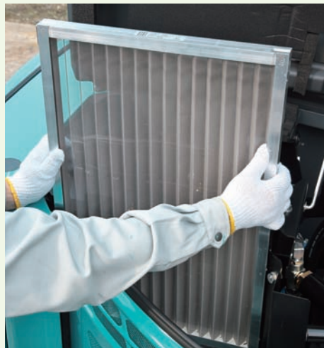
30-mesh means that there are 30 holes formed by horizontal and vertical wires in every square inch of filter.
