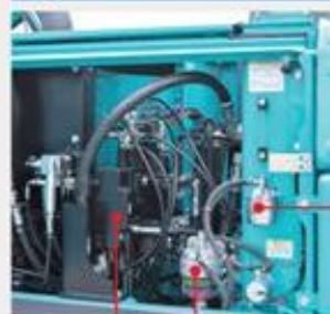
Pre fuel filter (with built-in water separator)
